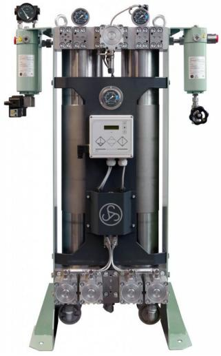
*Figure 3: Sauer USA Desiccant Dryer capable of operation up to 7250 psig.*
