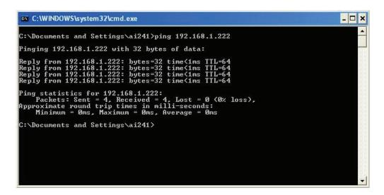
FIGURE 4-13. PING TEST SUCCESSFUL
