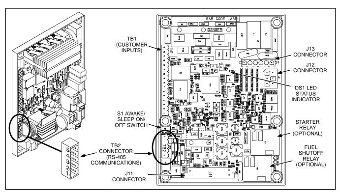
FIGURE 3-5. PCC1301 CONTROL BOARD WITH RS-485 COMMUNICATIONS PORT
