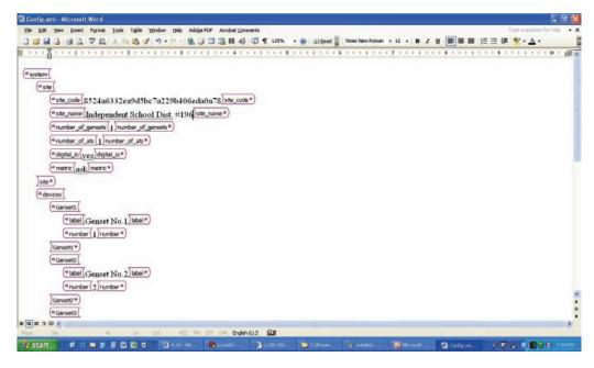
FIGURE 4-2. READY TO EDIT CONFIG.XML FILE
