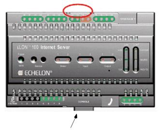
The locking tab is located below console port DB9
