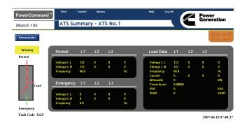
FIGURE 5-7. ATS SOURCE AND LOAD DATA
