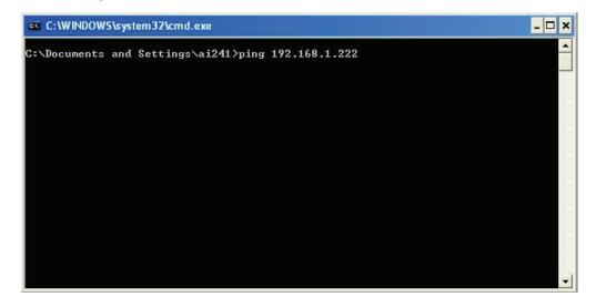
FIGURE 4-12. PINGING A DEVICE ON THE SUBNET
