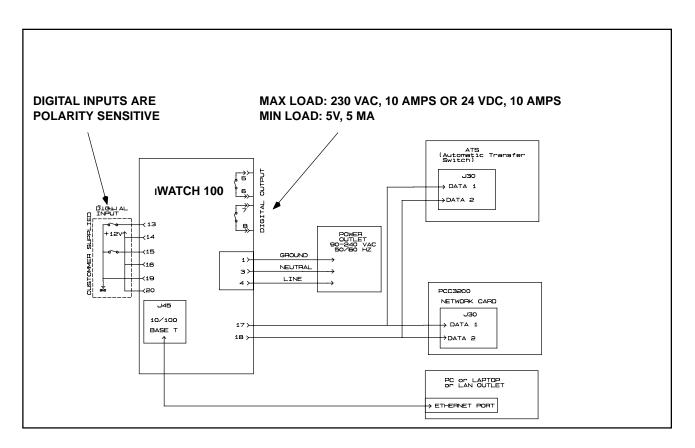
FIGURE 3-10. POWERCOMMAND IWATCH 100 WITH POWERCOMMAND 3200 CONTROL
