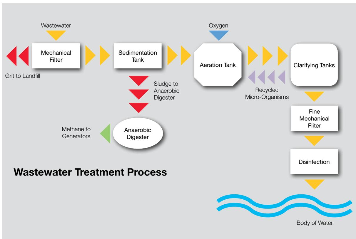
Wastewater exiting a home or commercial property is collected via a network of gravity-flow pipes and delivered to the wastewater treatment plant. Also called the sanitary sewer system, these pipes are kept physically separate from storm water collection and distribution, which is often discharged directly to a body of water without any treatment or processing. Here are the next steps that wastewater might go through in a modern plant:
