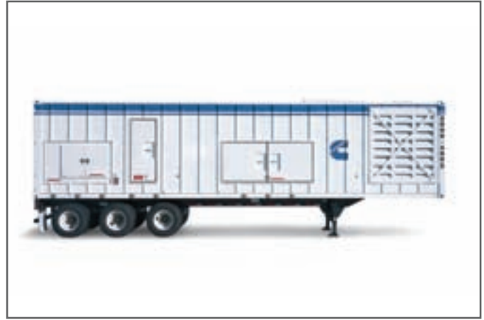
Each Rental Power unit was a stand-alone power station.
