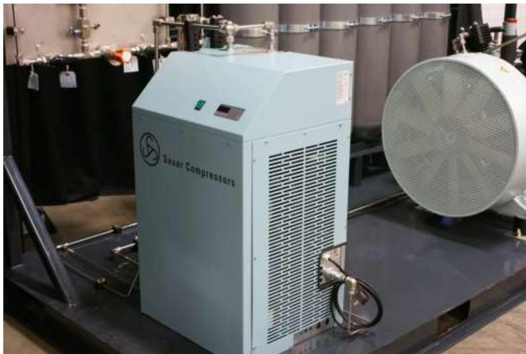
Figure 1: Sauer USA refrigerated dryer capable of operation up to 6000psi.
