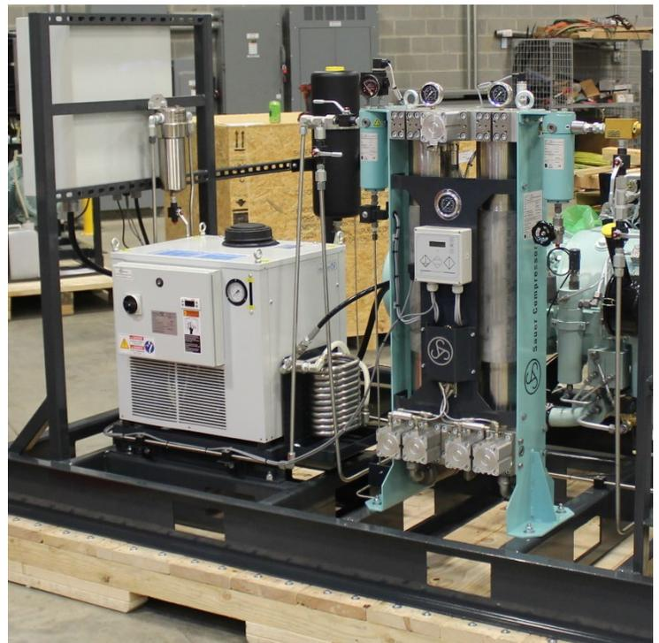
*Figure 2: Sauer USA desiccant dryer on a custom-engineered skid-mounted package.*
