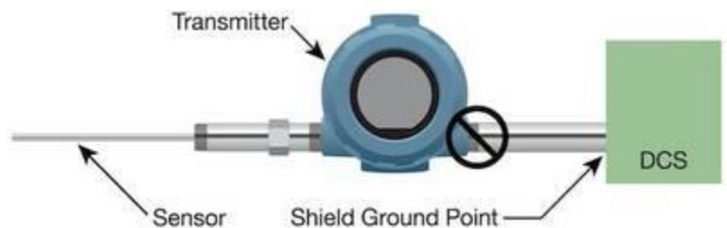
One additional tip: The instrument system ground should not be connected to a power wiring ground which can carry noise, surges, and spikes that could interfere with measurement signals and/or destroy transmitters. An instrument system ground must be a very low resistance path to an earth grounding rod or grid.
