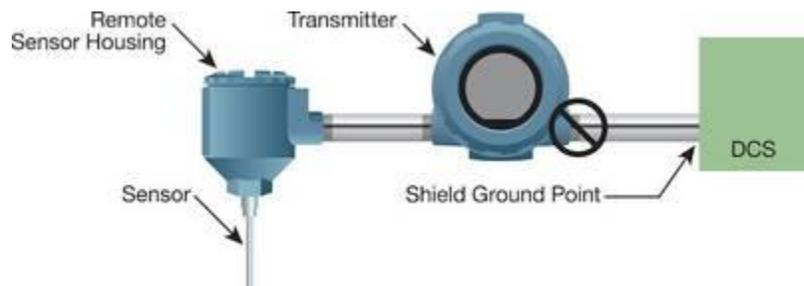
Option 3. Integral mount-Ground the signal wiring shield at the power supply end only to the instrument system ground ensuring that it is electrically isolated from the transmitter housing and all other field equipment. This is used for integral mount installations. (See Figure 5.)
