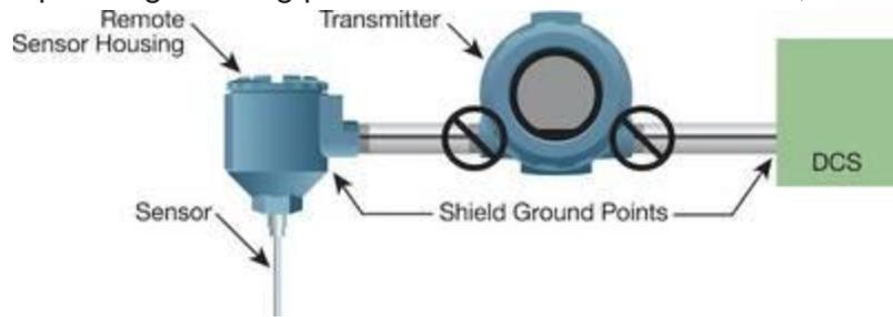
Option 2. Remote mount with a continuous shield-Connect the sensor shield only to the signal cable shield and ensure that it is electrically isolated from the transmitter and all other field equipment. Alternatively, connect the signal cable shield to instrument system ground only at the power supply end.
