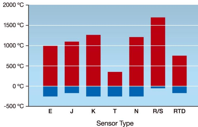
2. What is your required sensor accuracy? Determining the level of accuracy needed is also an important factor in the selection process. In general, RTDs are more accurate than TCs, and wire-wound RTDs are more accurate than thin-film RTDs. Assuming there are no other factors driving the selection of one technology over the other, this guideline will help you find the most accurate sensor technology.
