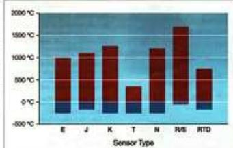
Thermocouples come in a variety of types determined by the combination of wire types. Most types have a higher temperature limit than an RTD.
