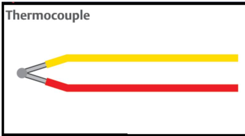
T/Cs have heavy gauge wire construction for durability, and therefore can withstand high vibration. The following chart compares the key sensor characteristics.
