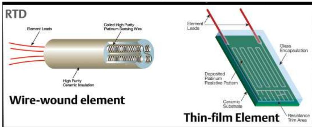
**Wire-wound RTDs** are manufactured either by winding the resistive wire around a ceramic mandrel or by winding it in a helical shape supported in a ceramic sheath – hence the name wire-wound.
